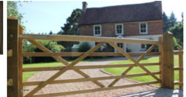
Gates are 1.27m high overall. Top rail 100mm x 75mm, under rail and cross braces 75mm x 25mm. Hanging and slam stiles (rounded top) 100mm x 75mm (nominal sizes), with both stiles drilled to allow gates to be hung on the left or the right. Supplied in natural Jakcure® treated finish.
