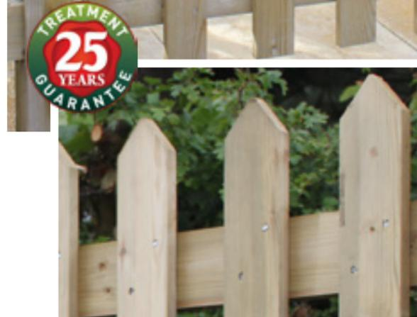
Pales are nominal 75mm x 22mm section, (70mm x 19mm planed finished size) planed with pointed or rounded tops with pale tops machined. When calculating materials required, you will need one post for every 2.28m plus one extra for the end of the run. There are 14 pales per bay. Each bay is backed by two 2ex 87 x 38mm nominal rails.
