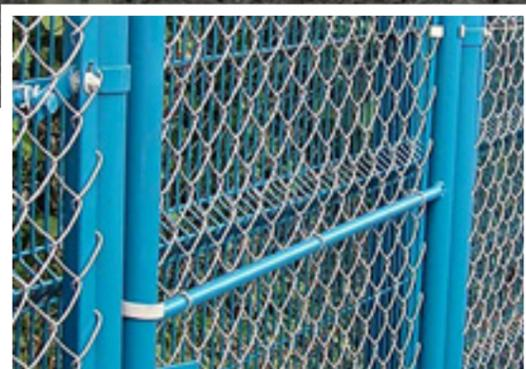
They are right or left hand hanging and clad with galvanised coated chain link, also available in a green finish. The framing is made from 42mm diameter galvanised tube. The gates come ready for hanging, complete with hinge pins, and bolts for attaching to the end strainer.
