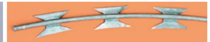
Features: A wide central steel band which provides additional rigidity to the coil. The blades are substantial and effective: 20mm tip to tip. 35mm centre to centre.
