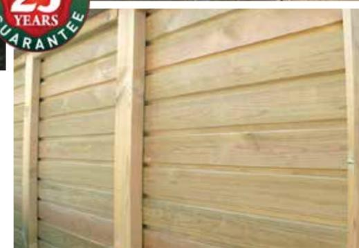
They feature a mortice and tenon jointed frame for extra strength while the infill is constructed using horizontal Tongue and Groove Effect boards. The centre of the panel is given additional support with one 70mm wide rail for heights up to 1.22m, and two rails for heights of 1.52m and above.
