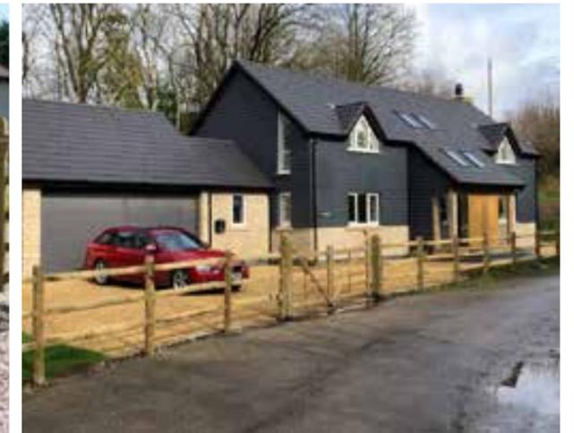
Allow one post for every 1.85m of fence, plus one for the end of the run.
