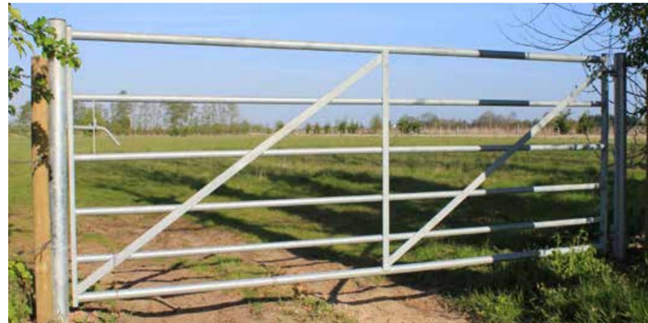
**Specification:** Gates are 1.15m high. Hanging stile of 50mm x 25mm box section. Slam stile of 50mm x 25mm box section. Top and bottom rails 41.5mm tube, with middle rails 32mm tube. Fittings include adjustable hinges and padlockable sliding latch. Also available with welded mesh cladding, (600mm high x 50mm x 50mm x 4mm) to the bottom part of the gate, please see below.
