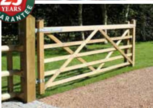
All timber used throughout is superior quality planed Jakcure® treated softwood guaranteed for 25 years. Top bars are chamfered and both hanging and slam stiles are drilled to allow gates to be hung on the left or right. Rail and brace crossings are bolted with stainless steel bolts. The gates are cross braced for extra strength and all joints are morticed and tenoned.
