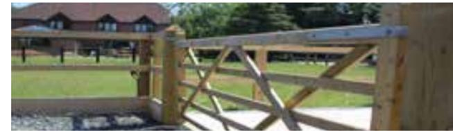
Gates are 1.27m high overall. Top rail 100mm x 75mm, under rail and cross braces 75mm x 25mm. Hanging and slam stiles (rounded top) 100mm x 75mm (nominal sizes), with both stiles drilled to allow gates to be hung on the left or the right. Supplied in natural Jakcure® treated finish.
