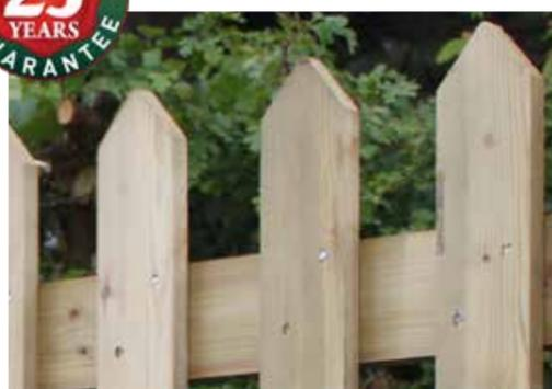
Pales are nominal 75mm x 22mm section, (70mm x 19mm planed finished size) planed with pointed or rounded tops with pale tops machined. When calculating materials required, you will need one post for every 2.28m plus one extra for the end of the run. There are 14 pales per bay. Each bay is backed by two 2x 87 x 38mm nominal rails.
