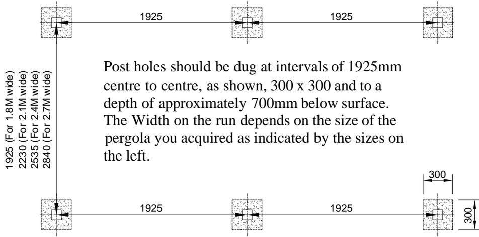
Post holes should be dug at intervals of 1925mm centre to centre, as shown, 300 x 300 and to a depth of approximately 700mm below surface. The Width on the run depends on the size of the pergola you acquired as indicated by the sizes on the left.
