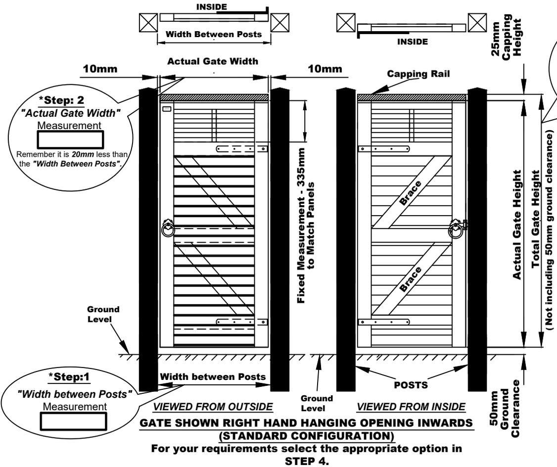
For gate's with "Actual Gate Height" 1.35m or less, the gates are manufactured with single brace.
