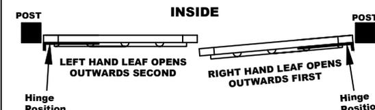
d. For Gates with Left Hand Gate opening outwards first
