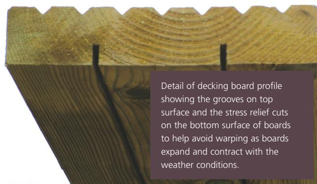
Detail of decking board profile showing the grooves on top surface and the stress relief cuts on the bottom surface of boards to help avoid warping as boards expand and contract with the weather conditions.
